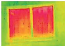
Heat energy is transferred from homes by conduction through the walls, floor, roof and windows.
